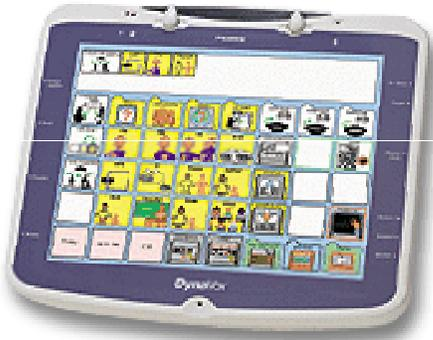
The **DynaVox 3100 by DynaVox Systems** is an AAC device with dynamic display and powerful communication software.
