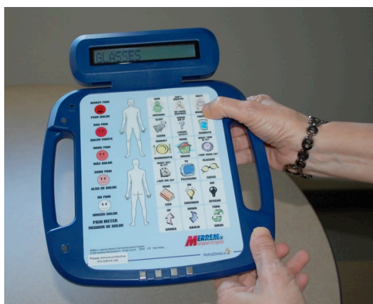
Caption: Demonstrating the back of the Zam Communicator with LCD screen displaying the text "glasses"
