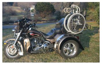
Here is a wheelchair lift on a custom trike. The wheelchair is attached to an arm on a track that lifts it onto the fender. The lift gives riders wheels on their bike or in their chair and is the product of The Freedom Track, www.freedom-track.com.
